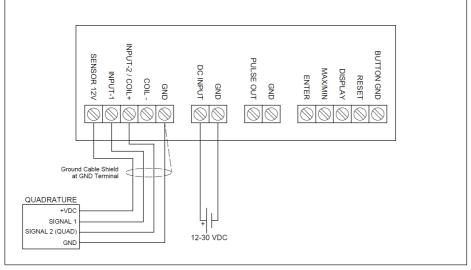
Note: If negative flow is displayed during "forward flow" conditions, swap the wiring connections for signal 1 and signal 2 (Quad).
