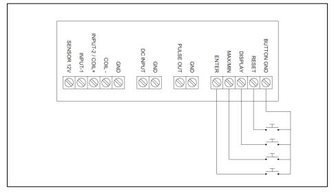
External switches may be connected to the RT40 display to allow remote access to button functions, or to allow use of heavy industrial push buttons in environments where the standard switches may break or wear. Momentary normally open (NO) switches MUST always be used.
