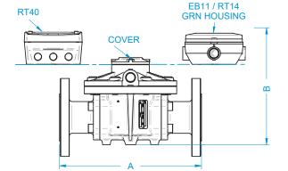
OM040: Ø6.3 in. (160 mm) OM050: Ø7.1 in. (180 mm) OM015: Ø4.3 in. (110 mm) OM025: Ø4.7 in. (120 mm)
