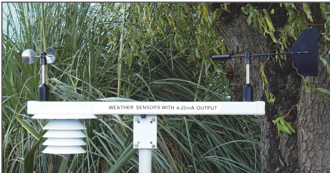
TBar with Wind Speed, Wind Direction plus Solar Radiation Shield
