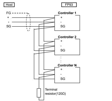
Note1: In the case of RS-485, provide it with the attached terminal resistor of 1/2W,  $120\Omega$  across terminals + and if necessary. Nevertheless, it should be provided to only the last controller. If two or more controllers are provided with terminal resistors, correct operation cannot be guaranteed.
