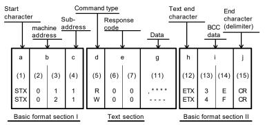
• The basic format portions I and II are common to commands (R), write commands (W) and responses. Nonetless, in BCC data of i (13, 14) operation result data is inserted each time.
