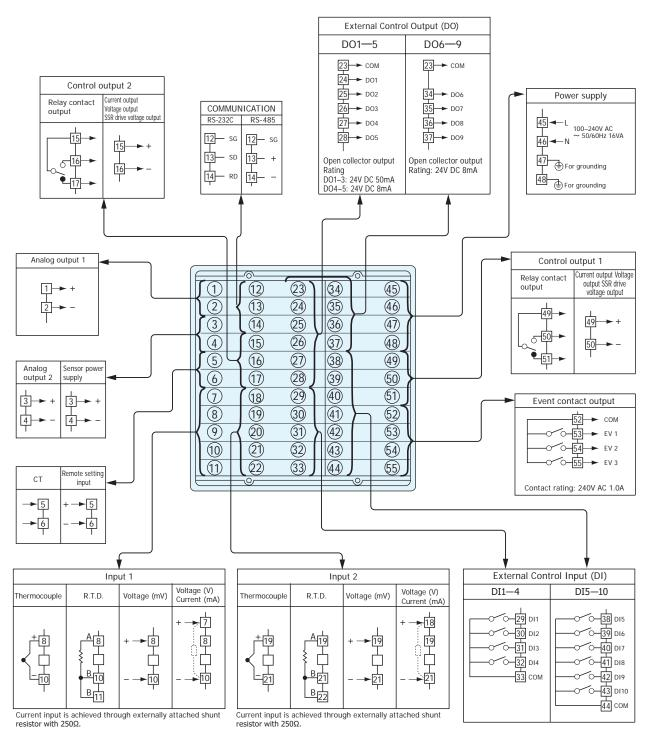
Crimp-type terminals fit M3 screws.
