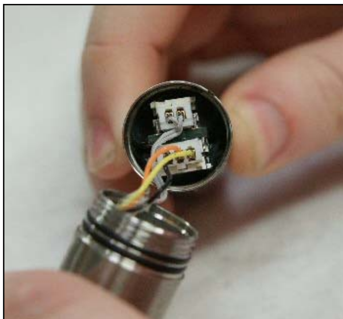
Fig 2: Identify the Battery and Communications wires.
