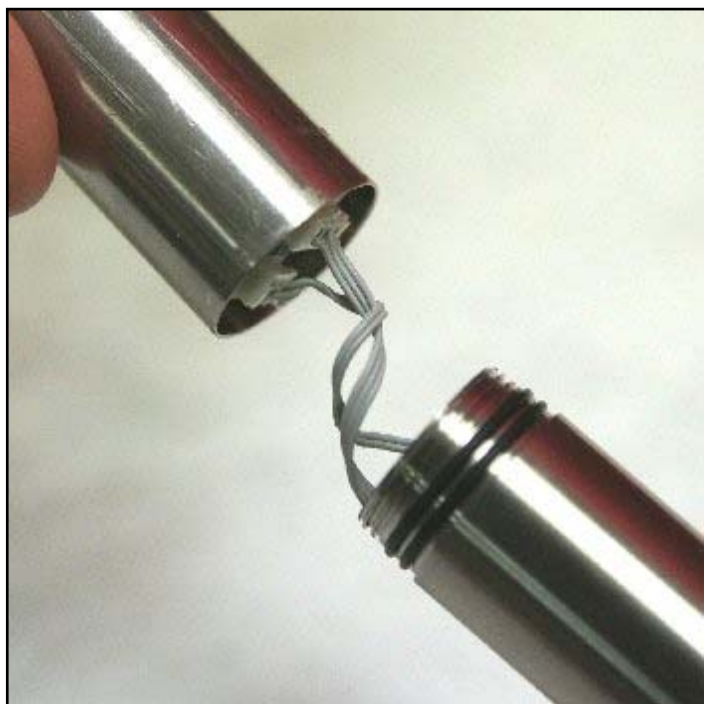
Fig 7: Pre-twist the wires Anti-clockwise.
