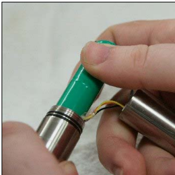
Fig 4: Withdraw the old battery.
