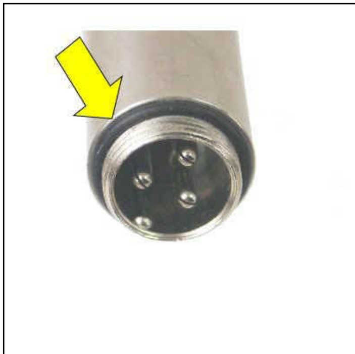
Fig 9: Check Communications Socket O-ring and replace if damaged.
