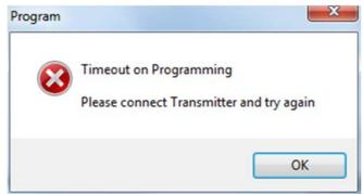
The software closes the connection, connect the transmitter to the computer again then click Connect and do the programming operation again.
