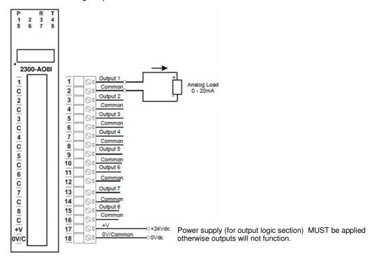
**Note:** Logic power output (terminals 17 & 18) range 24Vdc. The logic power supply output must be isolated and completely separate to the power supply that powers the 2300-AO8I on terminals 81 & 82. Failure to do so will cause the comms to stop.
