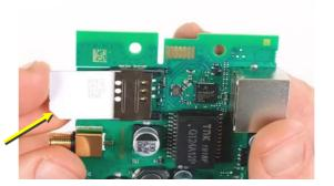
Carefully slide the circuit board back into the case and screw the case back to together again.
