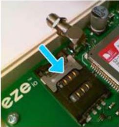
Slide the metal latch down to release hinged lid.
