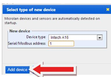
Next, enter the 'Serial/ModBus address', which must be set to the same number used in the 2400-A16 as well. See page 8 <<
