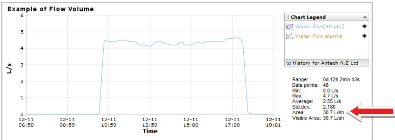
If the data shows L/s as on this graph, the 'Area' unit (volume) becomes L/s \* hours, so that eliminates the time component but you need to multiply by 3600 (seconds in an hour).
