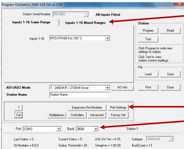
Configure the required input channel settings as shown. If all inputs being used are the same type, use the 'Inputs 1-16 Same Range' tab. If there are different input types being used, use the 'Inputs 1-16 Mixed Ranges' tab and configure each input as required.
