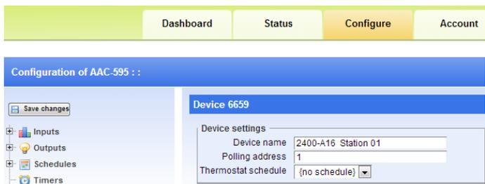
Remember that if two or more 2400-A16's are connected to the same ezeio™ Controller, the 2400-A16 '**Address**' and corresponding eze '**Polling address**' for each individual 2400-A16 must be set to a different number. **Never use the same number twice.**
