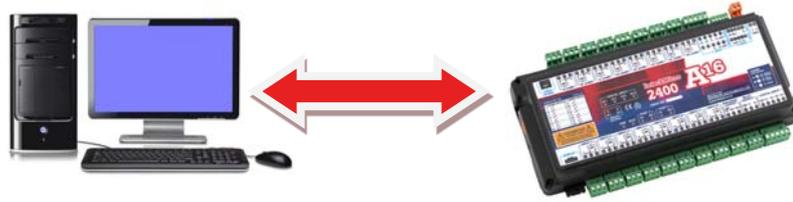
Connect the 2400-A16 to a computer as covered at the bottom of page 16 in the '**2400-A16 Installation Guide**'. If you do not already have a copy of the 'Intech Micro Station Programmer Software', download and install from this link: [www.intech.co.nz/downloads/Install-StationProgrammer.html](http://www.intech.co.nz/downloads/Install-StationProgrammer.html)
