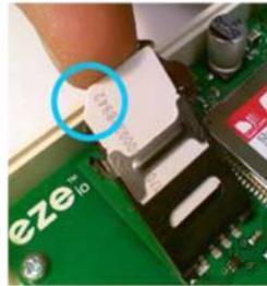
Insert SIM card into the lid. Orient cut corner top left.
