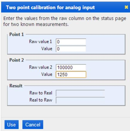
Point 1 is the zero point. As the flow meter range is 0~1000Hz, at zero flow, the Raw value and the flow meter value = 0.
