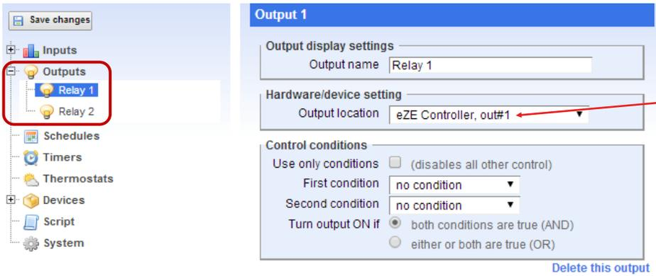
Select the actual hardware relay. In this example, it is the ezeio™ Controller, Relay Output 1.
