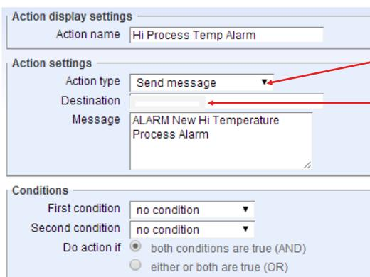
To configure sending an SMS text alarm or email alarm message, under 'Action type', select 'Send message'. Refer to **B** on page 24.
