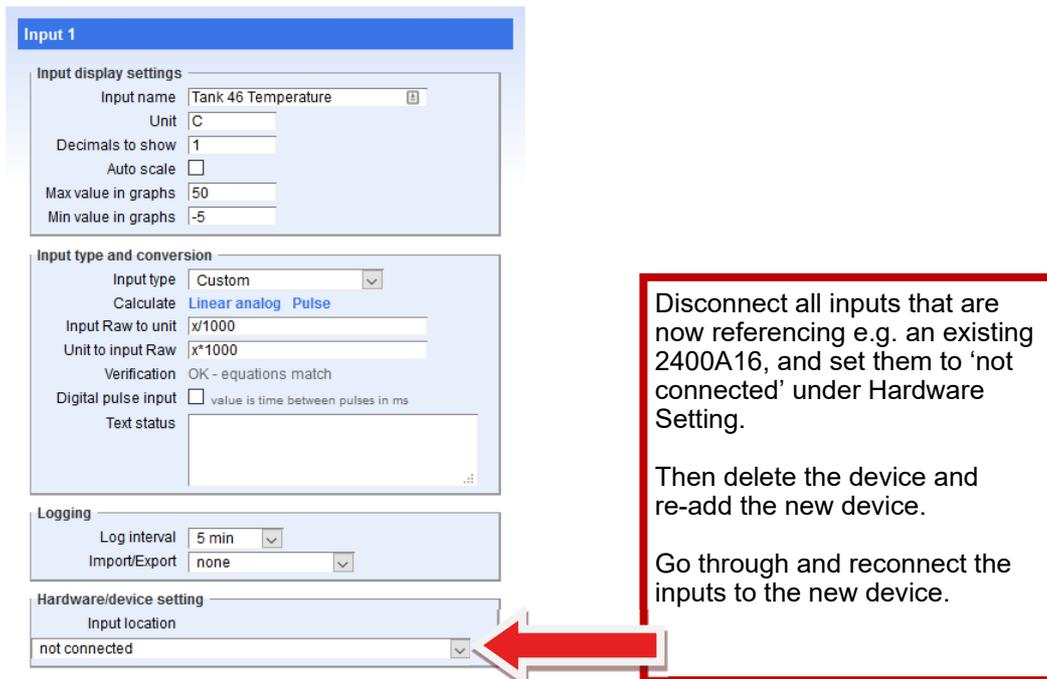
Disconnect all inputs that are now referencing e.g. an existing 2400A16, and set them to 'not connected' under Hardware Setting.
