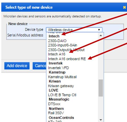
Under 'Device type', scroll down to the **Intech** section:
