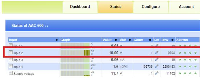
The screenshot shows the 'Status' tab of the AAC-600 controller. The title is 'Status of AAC-600 : :'. Below the title is a table with columns: Input, Graph, Value, Unit, Count, Set, Raw, and Alarms. The 'Input 2' row is highlighted with a red box. The 'Value' column for Input 2 shows '10.00' and the 'Unit' column shows 'V'. Other inputs include Input 1 (0.01 V), Input 3 (0.06 mA), Input 4 (1.6 m3/Hr), and Supply voltage (11.7 V).
