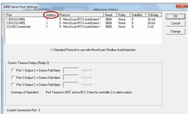
The **2400 Serial Port Settings** screen (left) displays the parameters the 2400-A16 should be set to, with special attention to the 'Address' which is referred to on the ezeio™ Controller as the 'Polling address'.
