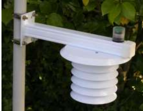
GP-HR-LB with Air Temp and Humidity sensors in Shield & Solar Radiation sensor.
