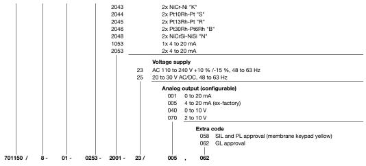
1. The first number on the measuring input means single probe "1" or double probe "2"
