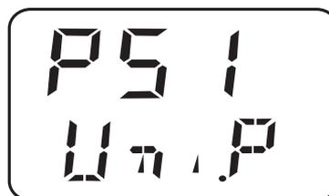
The measured pressure is shown in psi.
