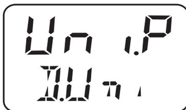
Uni.P = The measured value is displayed in the unit that was selected, see chapter 7.4 "Selecting the unit of the measured value (Uni.P)", page 31
