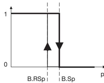
1 = Hysteresis of break contact (switching difference) = min. contact
