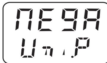
The measured pressure is shown in Megapascal (MPa).
