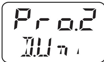
Pro.2 = The measured value is displayed as a percentage of the scaled measuring range, see chapter 7.8.1 "Setting the starting value of scaling (Sc.Lo)", page 38 and chapter 7.8.2 "Setting the final value of scaling (Sc.Hi)", page 39.
