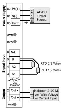
Note. All examples on RTD1 Sensor Break output will drive upscale & on RTD2 Sensor Break output will drive Downscale.
