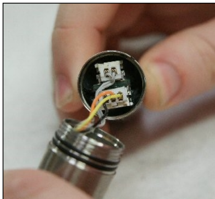
Fig 2: Identify the Battery and Communications wires.
