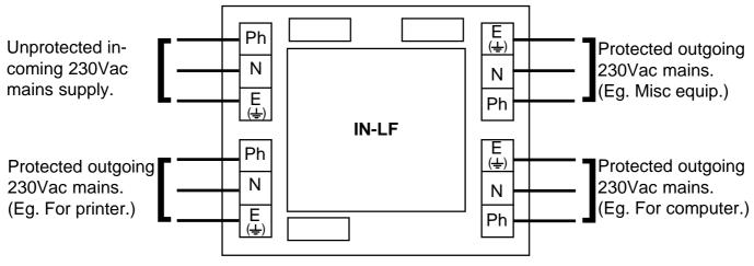
**Note:** All protected outgoing 230Vac mains are internally connected.
