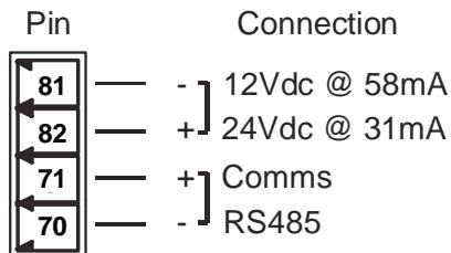
**Warning:** If the power/communication connections are reversed, the remote station may become faulty.
