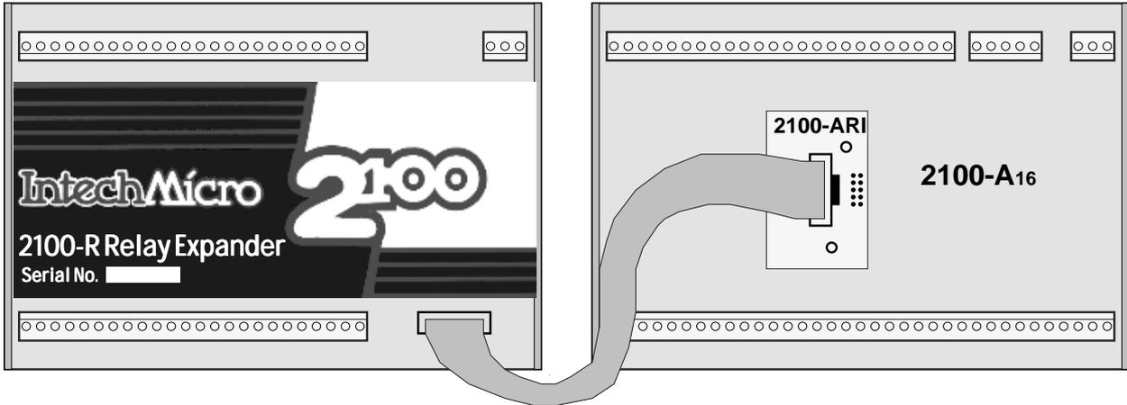
**WARNING:** The 2100-ARI is STATIC SENSITIVE. Only touch the edges of the PCB. Ensure standoffs lock firmly into the 2100-A<sub>16</sub> board.
