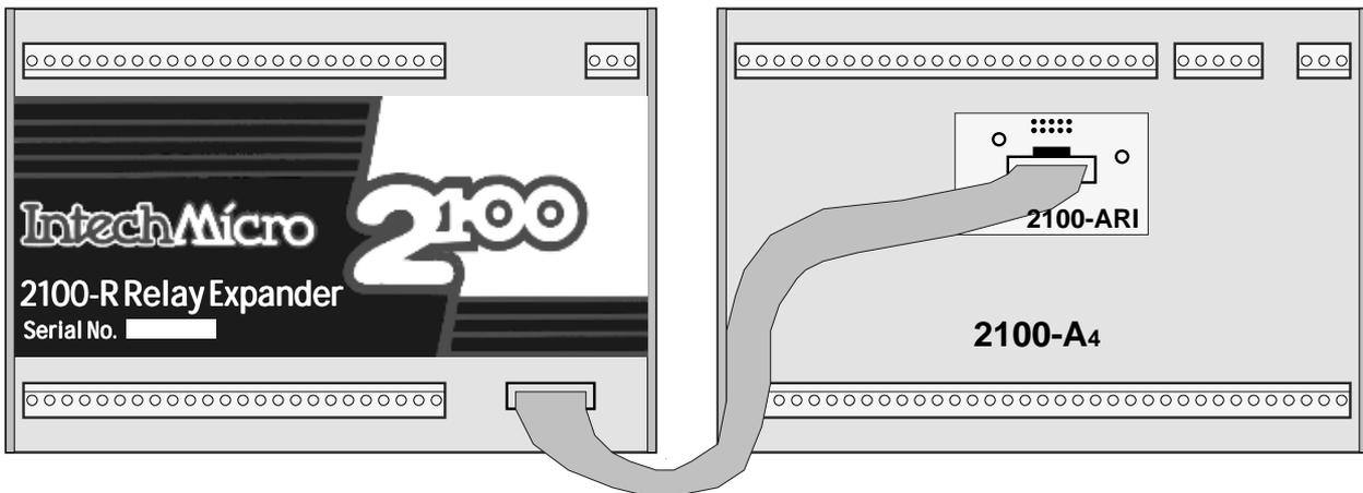
**WARNING:** The 2100-ARI is STATIC SENSITIVE. Only touch the edges of the PCB. Ensure standoffs lock firmly into the 2100-A4 board.
