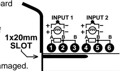
**2100-R with 2100-A<sub>16</sub> Relay Output Allocation for Single Action Controller.**
