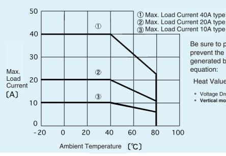
Be sure to provide enough ventilation to prevent the temperature increase. Heat generated by PAC04 is lead from following equation:
