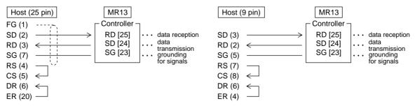
Note 1: Figures in () represent pin numbers of connector. Note 2: Figures in [] represent terminal numbers of MR13.
