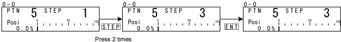
When "0" is set to the start step, that pattern is not executed. To execute control, set a value other than "0" to the start step.
