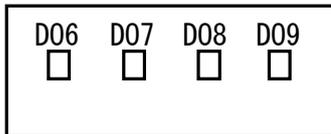
When DOx (x: 6 to 9) turns ON, □ is highlighted as ■. DO6 to DO9 are optional, then they are not displayed when they are not installed.
