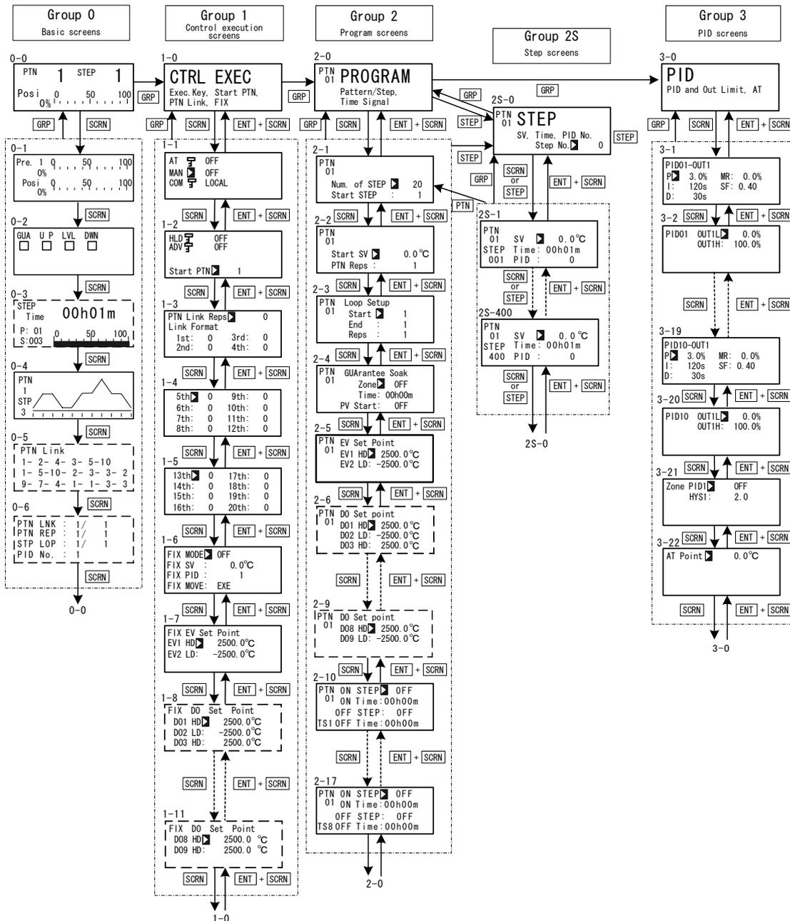
When the DISP key is pressed at a screen other than the 0-0 basic screen, the 0-0 basic screen is returned to.
