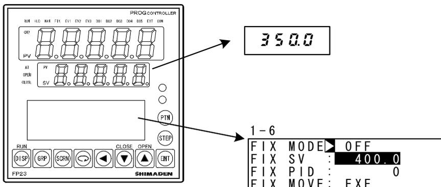
The white-inverted section indicates limiter over.
