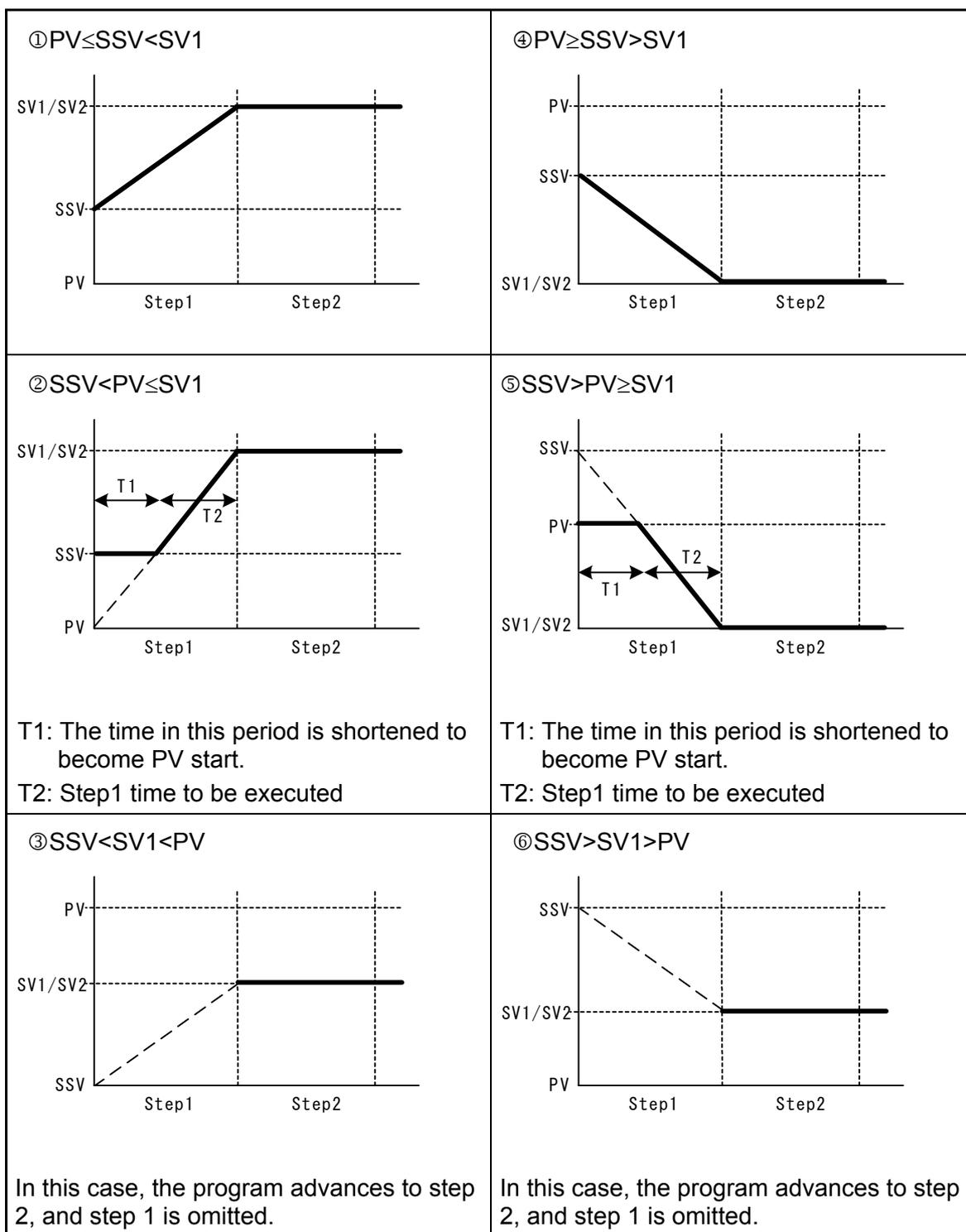
\*1 PV start is enabled only when the start step time is set to "00m01s" or more.
