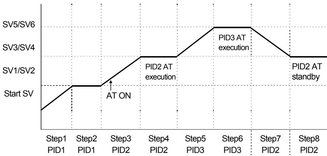
Step3 AT is in a standby state as the step is a ramp section. (AT LED lit)
