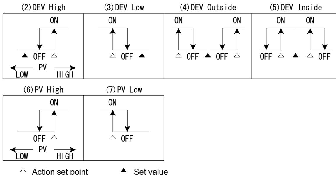
\* ON/OFF in the diagrams indicate operation mode. EVENT/DO output conforms to the setting (OPEN/CLOSE) of output characteristics.
