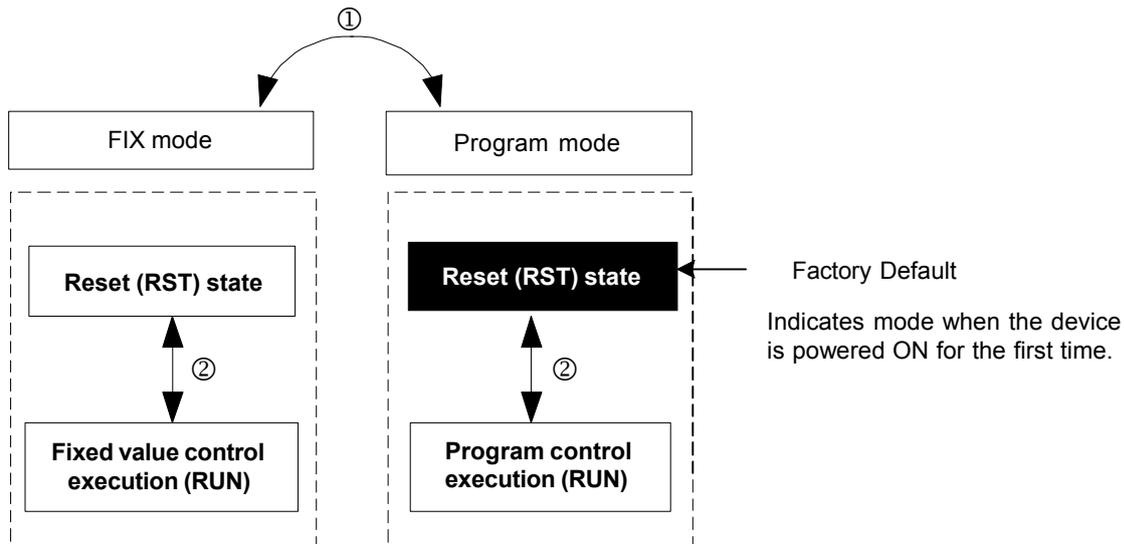
The control mode is switched by the FIX mode ON/OFF settings in the FIX MODE screen (No.1 to 6). The Mode switches to the FIX (fixed value) mode when ON is set, and to the Program mode when OFF is set.
