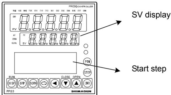
The following table shows the relationship between the start step No. in Reset state and the SV display.
