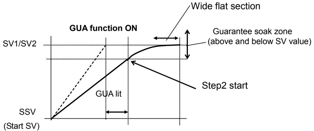
When the deviation between the step SV and PV of the flat step does not enter the guarantee soak zone when the ramp step switches to the flat step, the program does not move to the next step, and program execution stands by until this region is reached or the GUA time ends.
