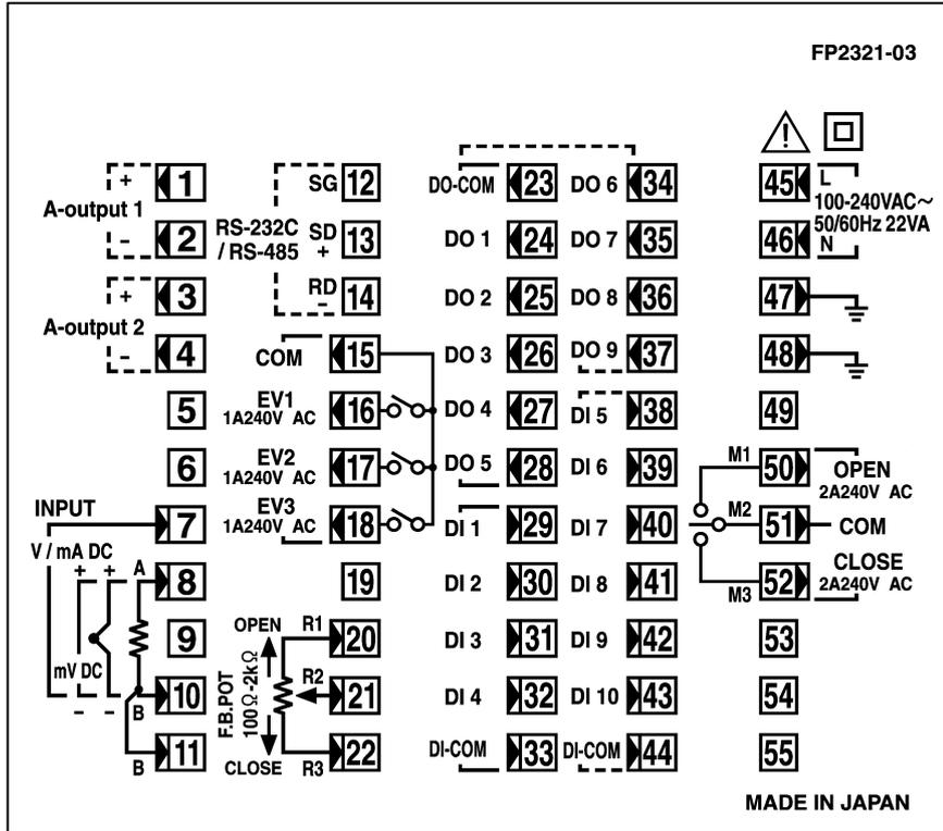
■ Combination of SSR output and contact output model
