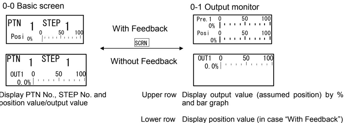
When used with Feedback, the output monitor displays OUT1 (control output) on the upper row and Posi (position value) on the lower row as a percentage (%) of the output value and a bar graph.
