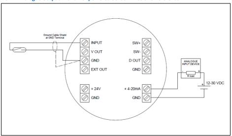
Notes: Shown here with Reed Switch input, Coil and Voltage Pulse inputs also suitable for this configuration.
