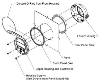
The rear enclosure of the instrument should be mounted behind the panel (as per diagram above) to protect the electronics module from damage and provide separation from any conductive components inside the panel/cabinet (this is compulsory for intrinsically safe installations)
