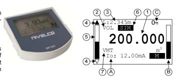
A., Calculated value of the output current. After the dimension, the mode of current output is indicated by inverse inscription:
