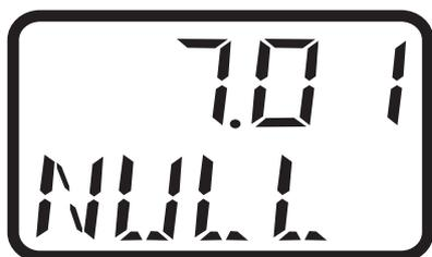
The calculated zero point of the measurement chain appears.
