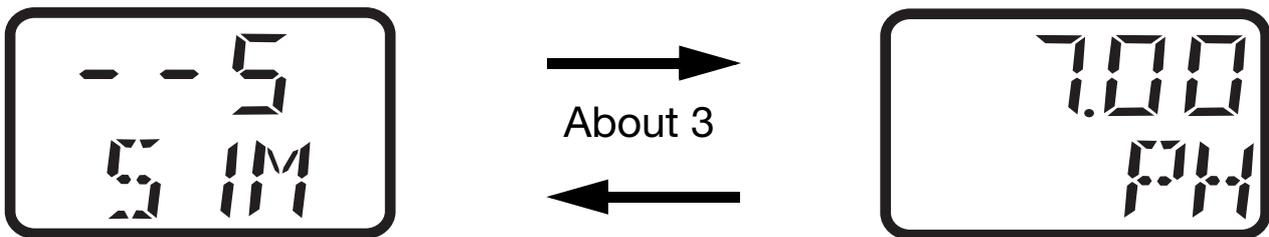
If one of the outputs is in manual mode, this is indicated in the change to process value display by an "S" or "-".
