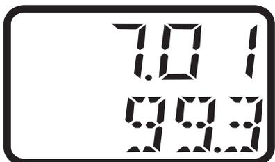
The calculated zero point (top line) and the calculated slope (bottom line) appear.
