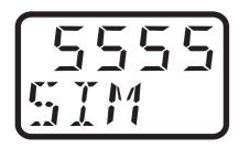
If one of the outputs is in manual mode, this will be indicated by displaying "S" or "-", in alternation with the actual value.
