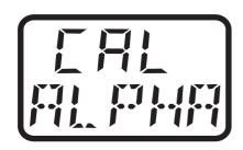
★ Confirm selection with P. continue with Chapter 9.4 "Calibrating the temperature coefficient using automatic temperature measurement", page 46 or Chapter 9.5 "Calibrating the temperature coefficient using manual temperature entry", page 49
