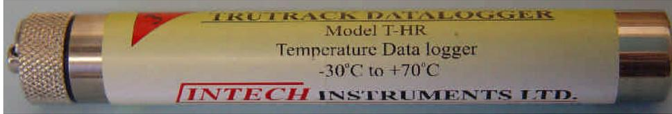
The T-HR is a small Single Channel High Resolution (12 bit) Temperature Datalogger with an internal sensor housed in a rugged 19.05mm 304 stainless steel case. The temperature sensor is mounted under a 0.6mm dome to give a relatively fast response time. Logging can be configured to; start on time, immediate start, stop when full, loop around (over write oldest data).
