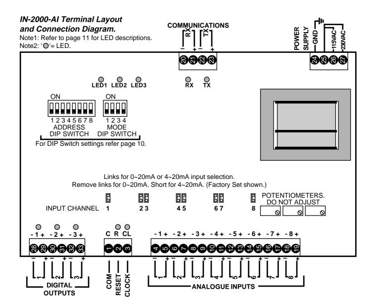
Connection Diagram of IN-2000-Al Open Collector Digital Outputs to 24VDC Relay Coils.
