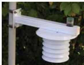
GP-HR-LB with Air Temp and Humidity sensors in Shield & Solar Radiation sensor.
